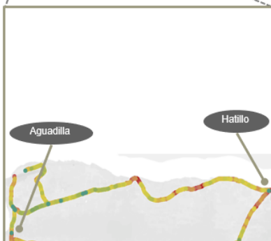
Good condition (IRI < 95) Fair condition (95 < IRI < 170) Poor condition (IRI > 170)
