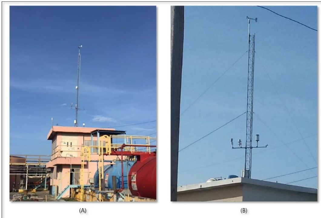
Figure 2. Onsite meteorological monitoring stations at the San Juan (A) and Aguirre (B) Power Plants.
