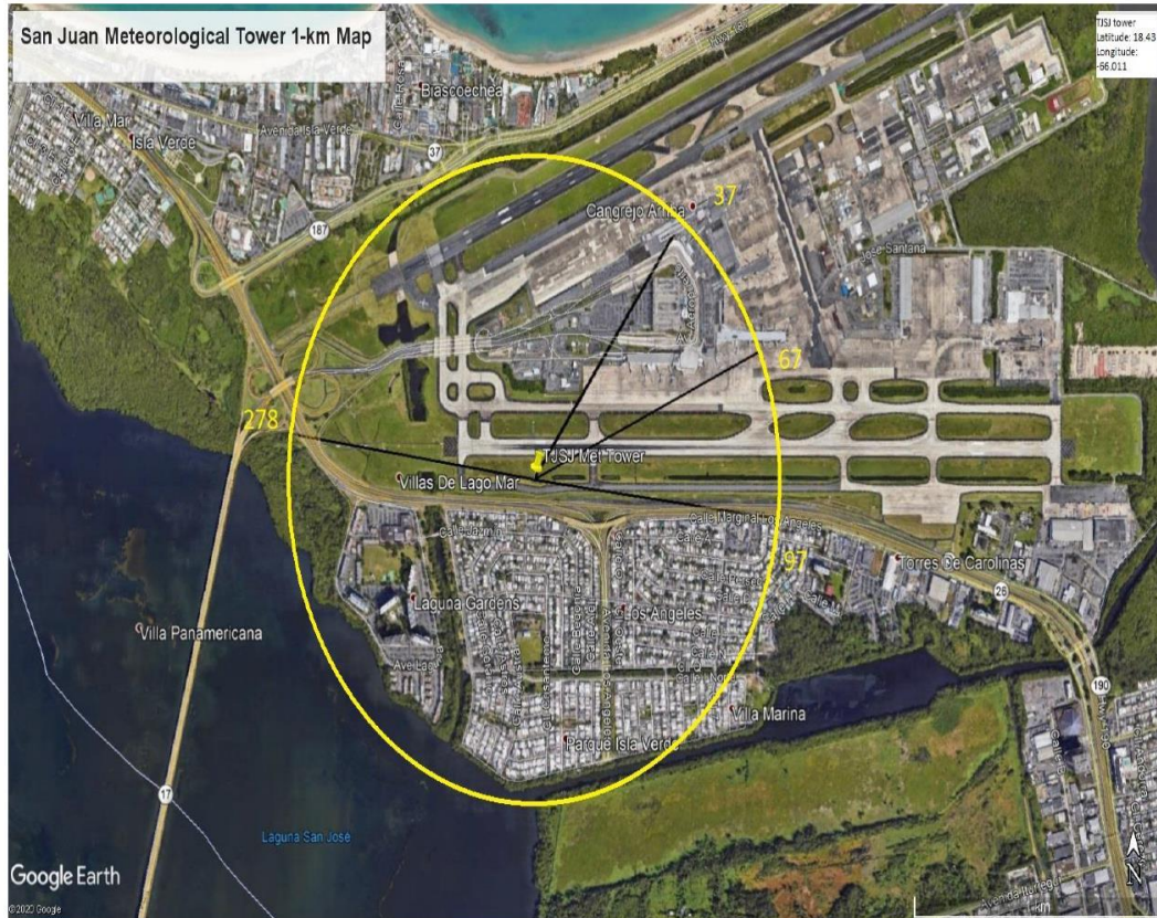
Figure 3.3 San Juan NWS tower 1-km radius circular area shown in yellow divided in circular sectors. Values shown are angles in degrees.
