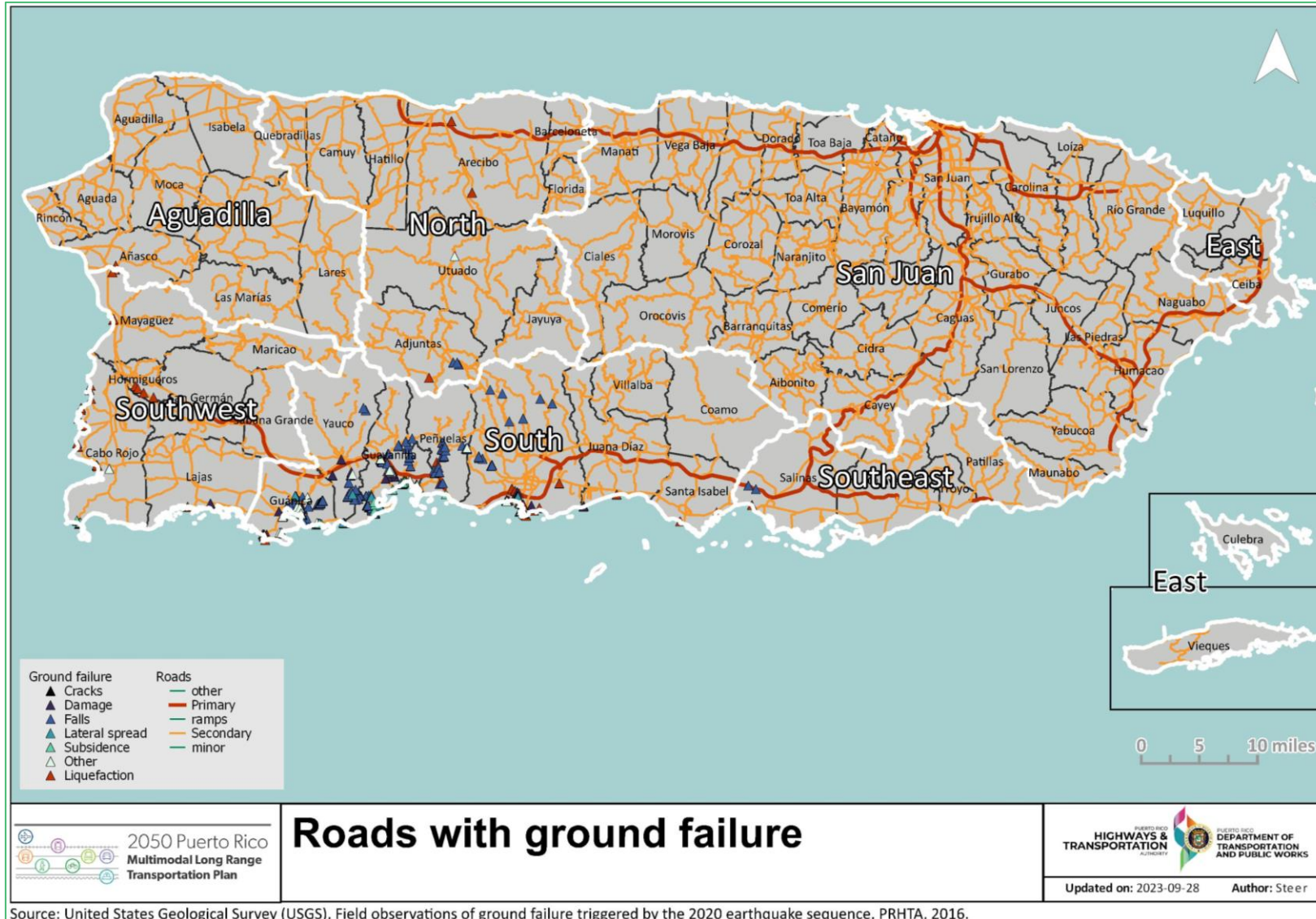
Figure 6.4: Principal Ground Failure Affections due to 2020 Earthquakes and Puerto Rico Road Network (Primary and Secondary Roads)
