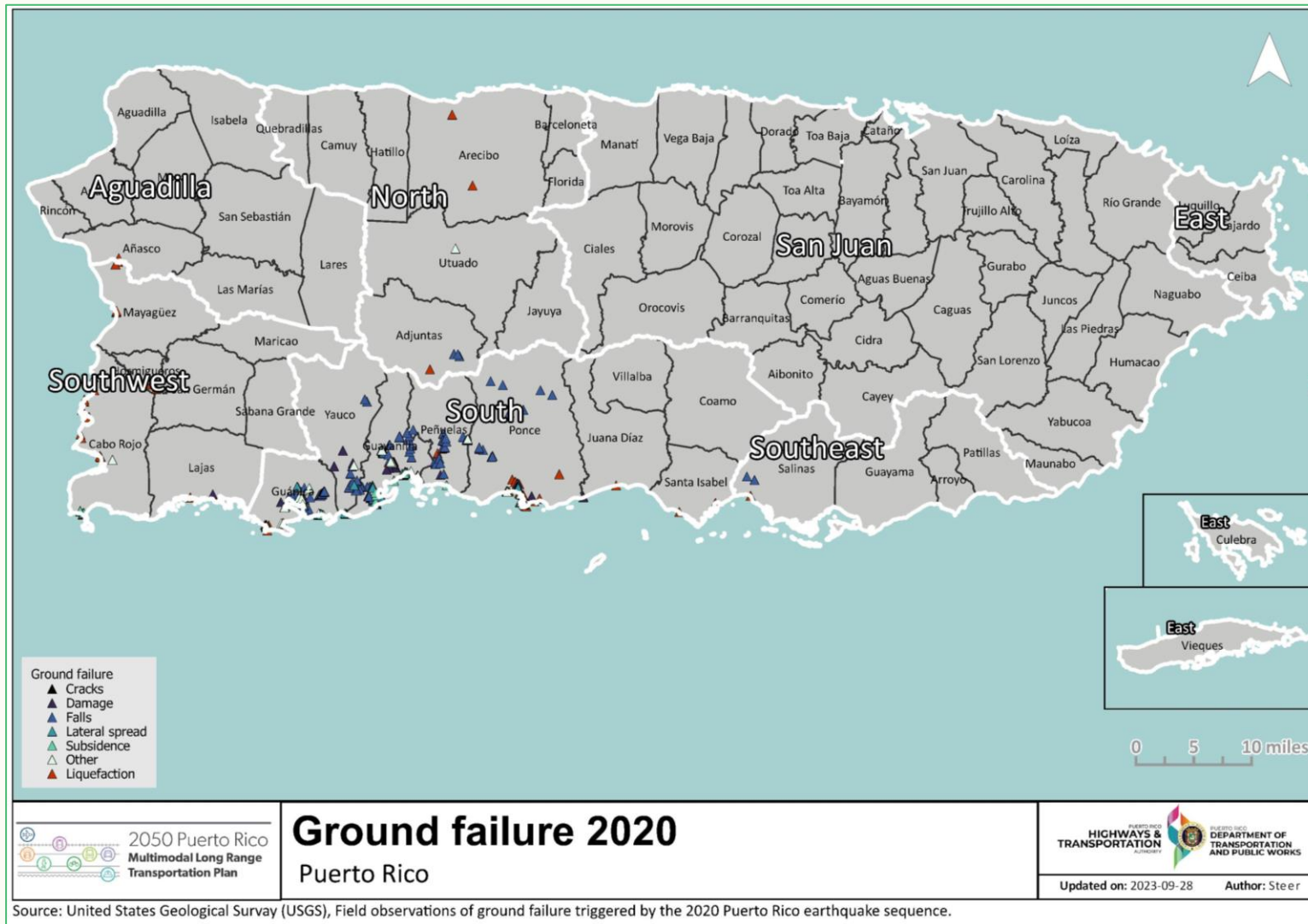
Figure 6.5: Principal Ground Failure Affections due to 2020 Earthquakes
