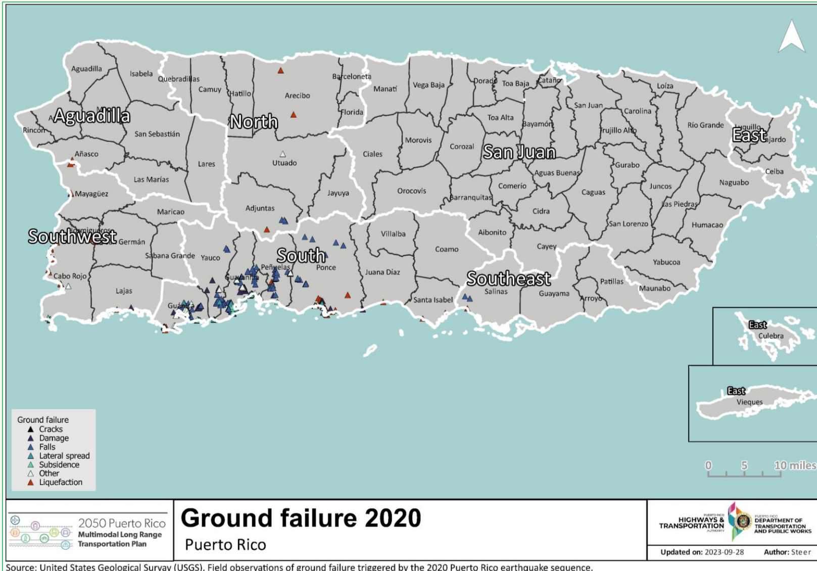
Figure 6.9: Principal Ground Failure Affections due to 2020 Earthquakes
