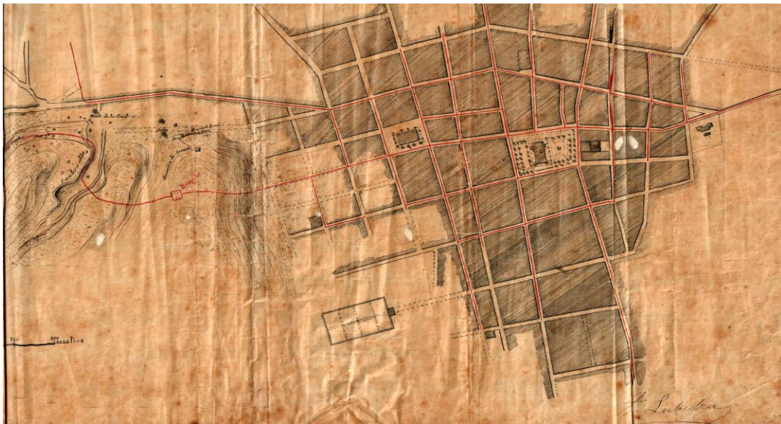
Figure 21. The upper image of the 1875 map prepared by Timoteo Lubelza shows the canal's route (in red) from the intake in the Portugués River, along Ponce's north outskirts, towards the deposit. The image below depicts the aqueduct's pipe network from the deposit throughout the city (also in red)
