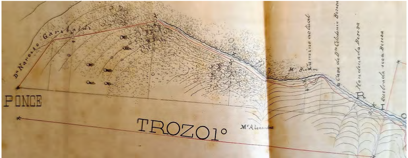
Figure 15. Partial view of Larrinaga's drawing of Carretera Núm. 6 first five kilometers. The proposed road, shown in red, two thousand meters after departing a point (Km. 0.0) in the property of Narciso Garibaldi would run in a northern direction along the eastern slopes of Rio Canas (in blue). This stretch was to end at Quebrada Besosa. Eventually, in the 1890s, Casilla #1 (see Section 7) was built in the proximity of kilometer 3.
