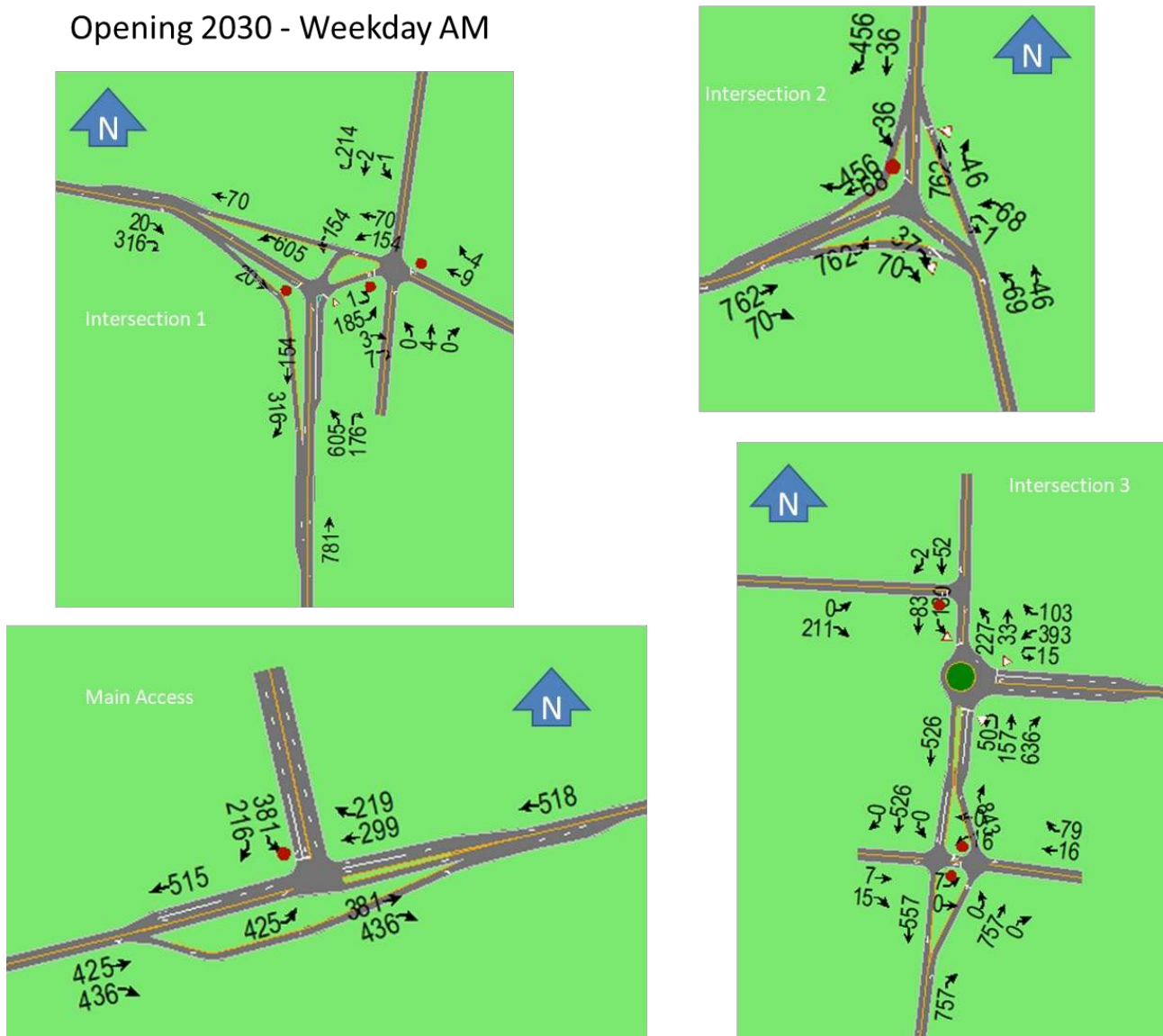
Figure 36 Peak Hour Volume for Opening Year 2030 – Thursday AM - Intersections 1 to 3 and Project's Main Access
