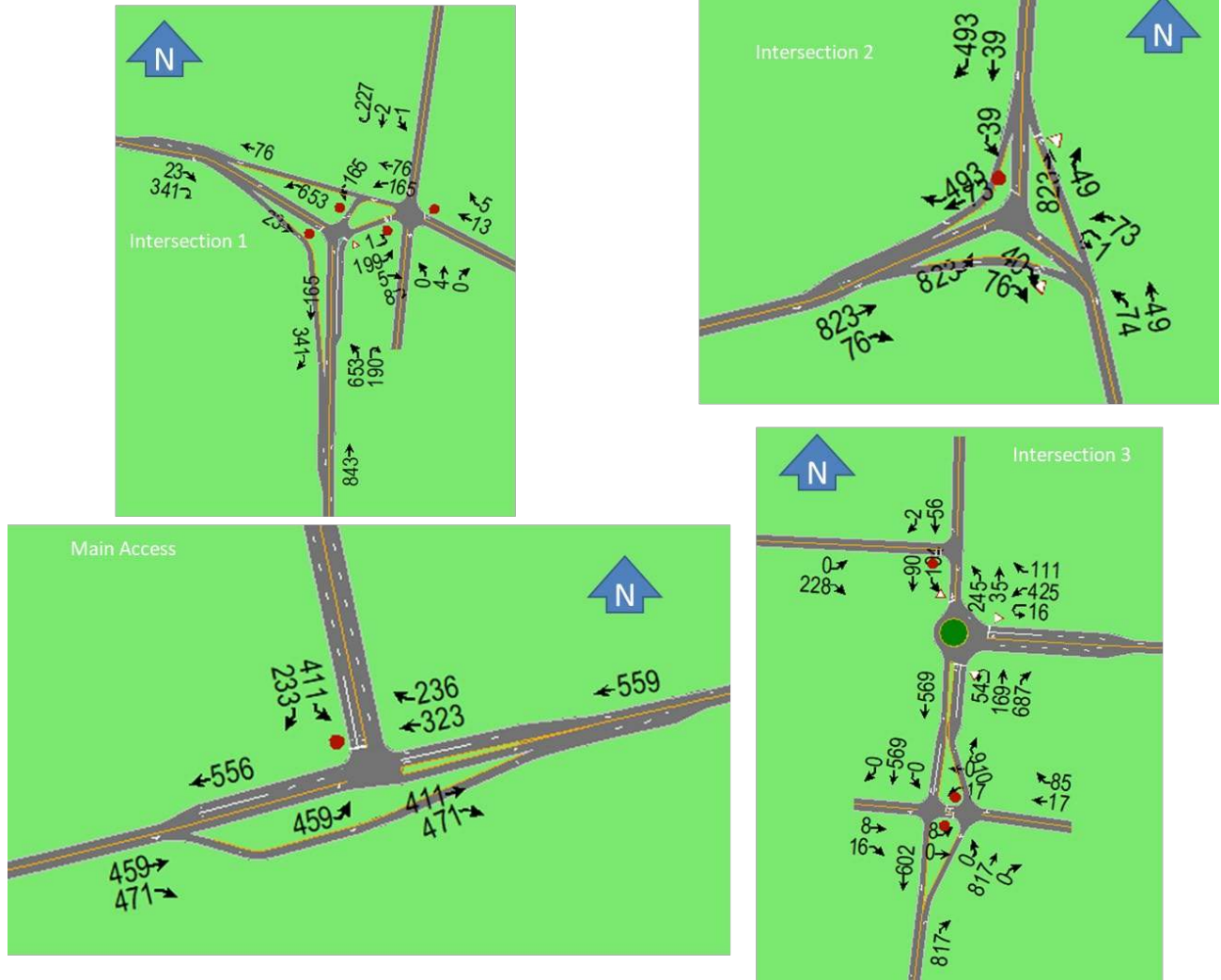
Figure 42 Peak Hour Volume for Opening Year 2035 – Thursday AM - Intersections 1 to 3 and Project's Main Access
