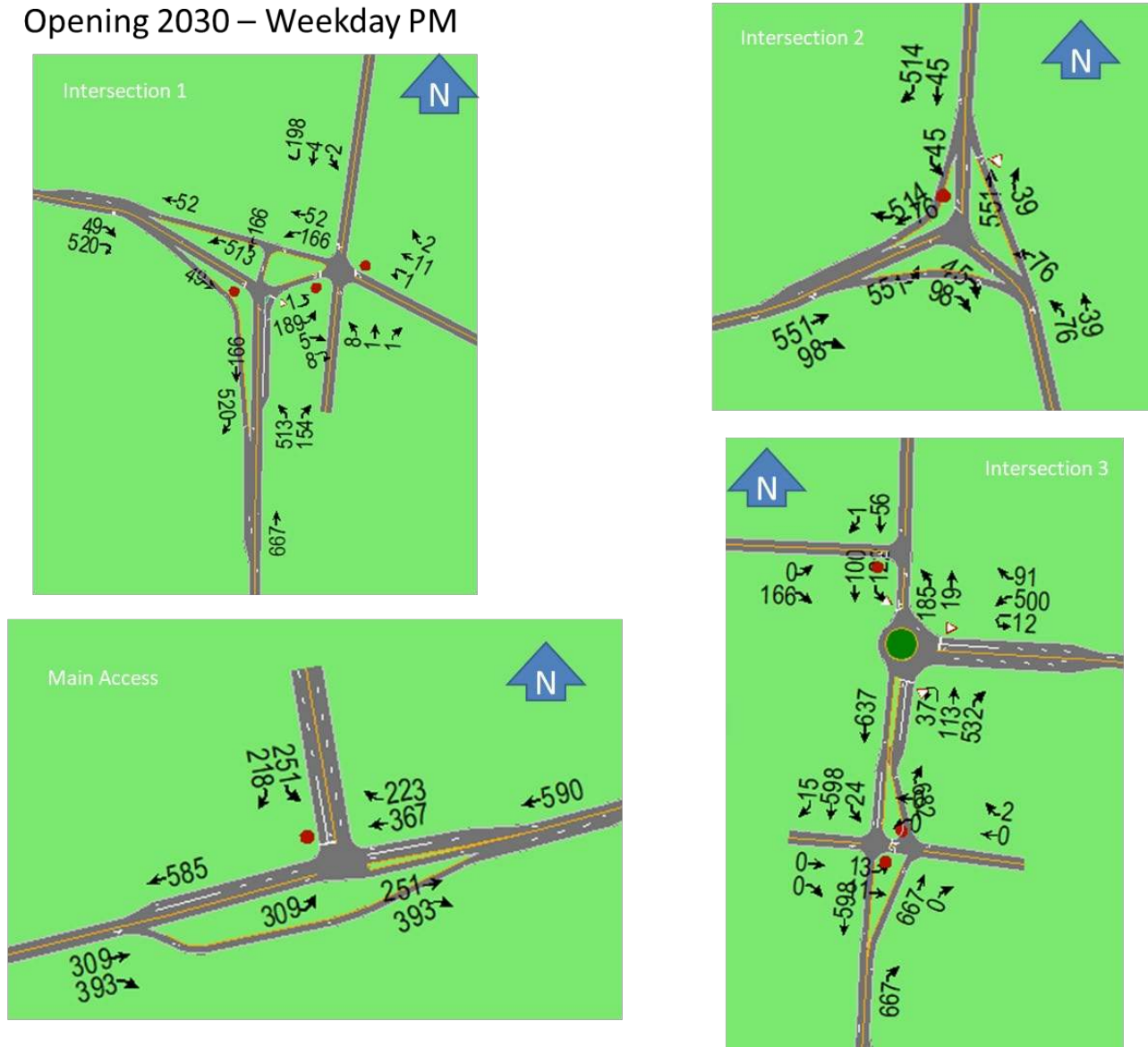
Figure 38 Peak Hour Volume for Opening Year 2030 – Thursday PM - Intersections 1 to 3 and Project's Main Access
