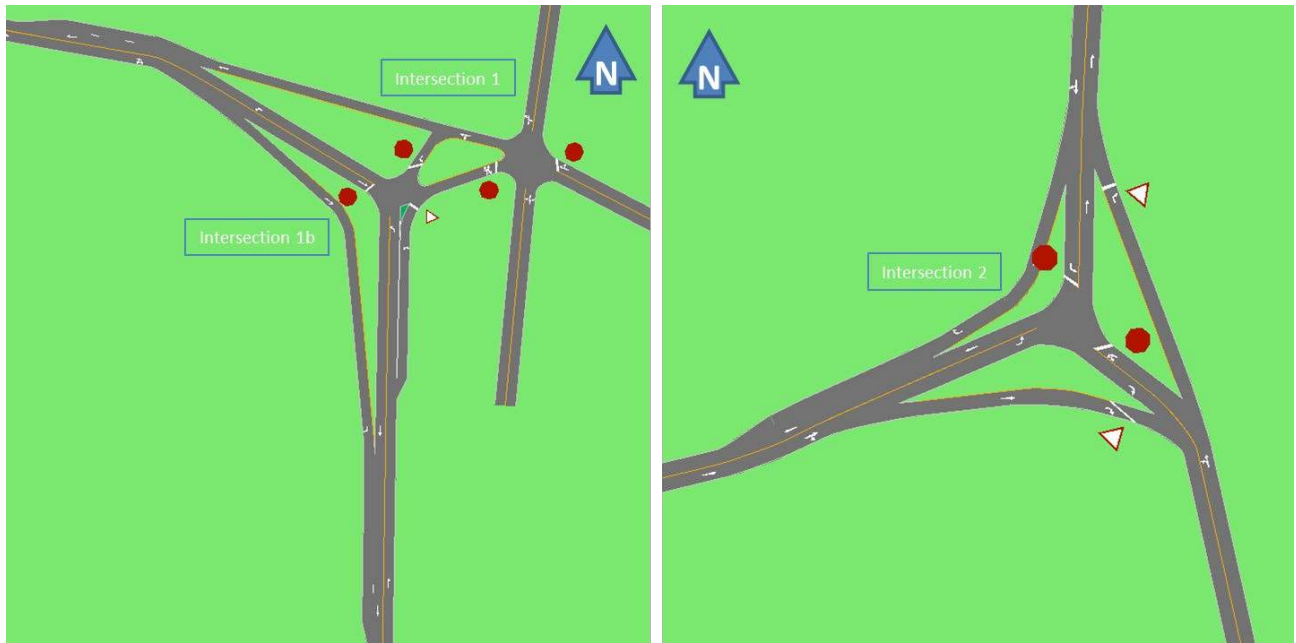
Figure 11 Existing Geometry of Intersections 1 and 2
