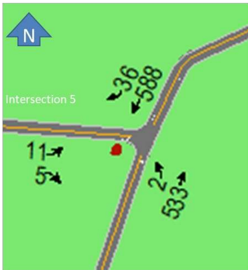
Figure 29 Peak Hour Volume for Opening Year 2028 – Saturday – Intersection 4, 5, Secondary Access, and BOH Access
