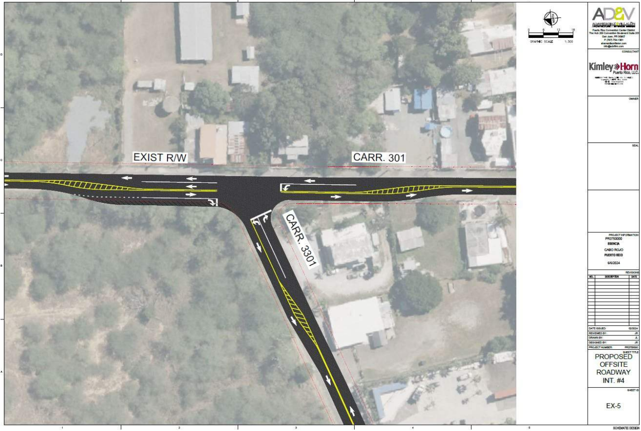
Figure 50 Conceptual Design for Intersection 4 Geometrical Improvements
