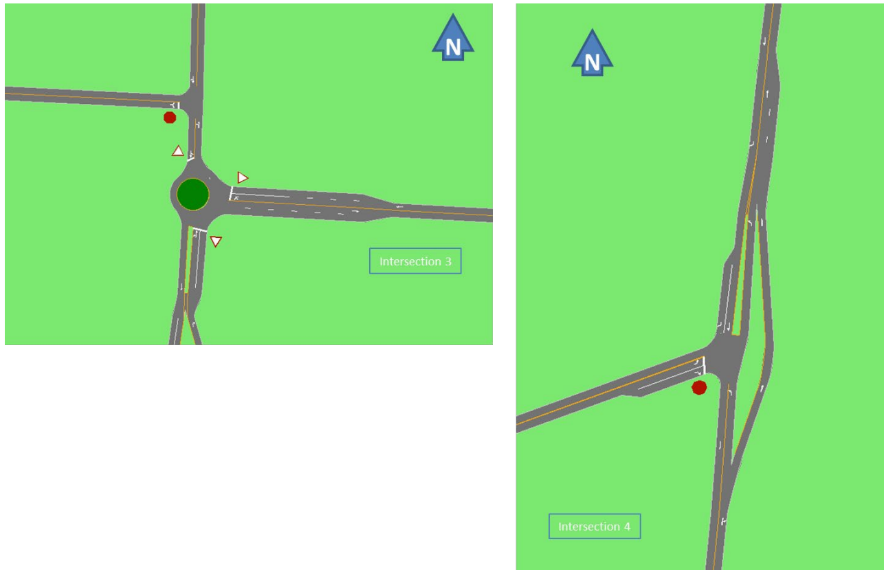
Figure 22 Proposed Geometry for Intersections 3 and 4
