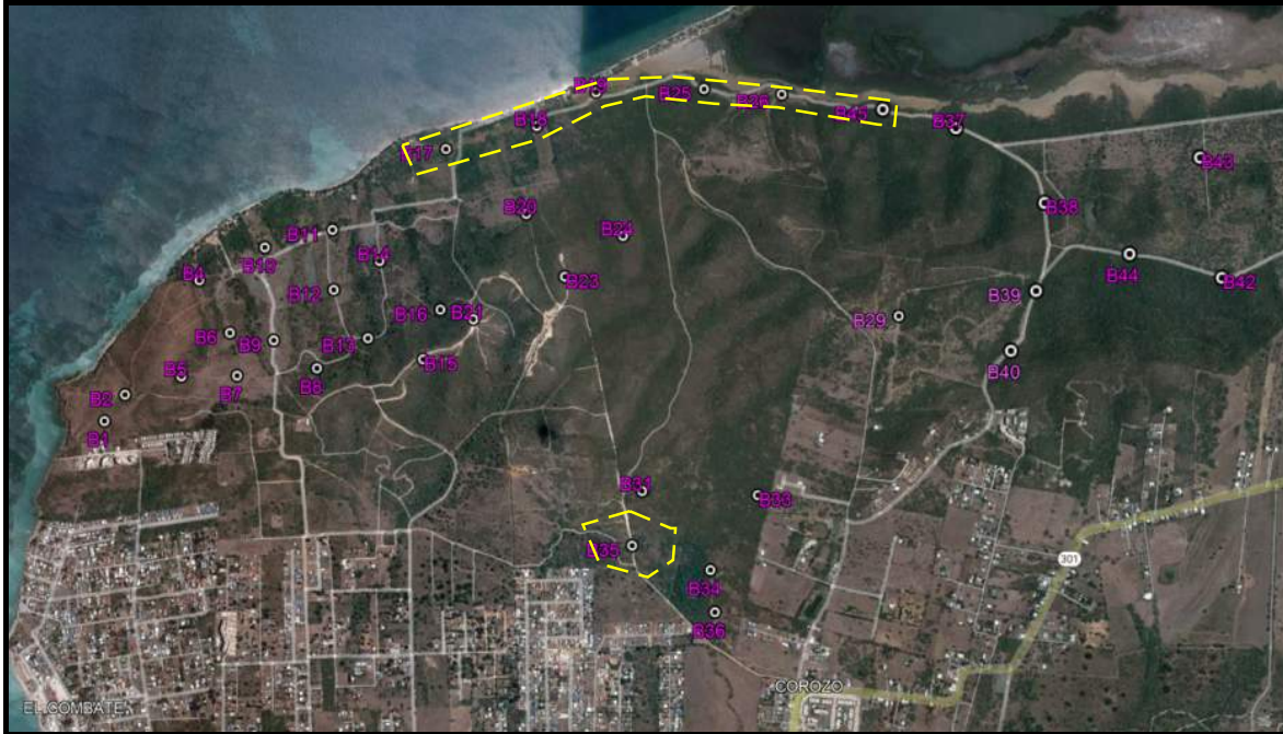
Figure 6. Dashed areas indicate the presence of alluvial soils of medium/marginal bearing capacity.
