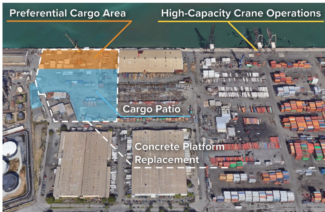
Figure 4. The concrete platform to be replaced, preferential cargo area and tenant cargo patio to be rehabilitated, and high-capacity crane operations are identified in this map of Wharf C.
