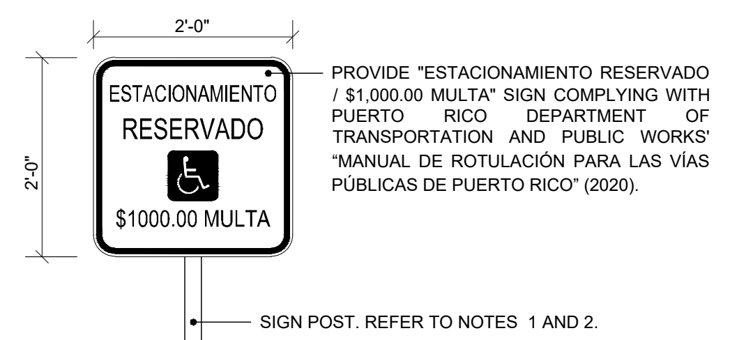
ACCESSIBLE PARKING SIGN DETAIL
