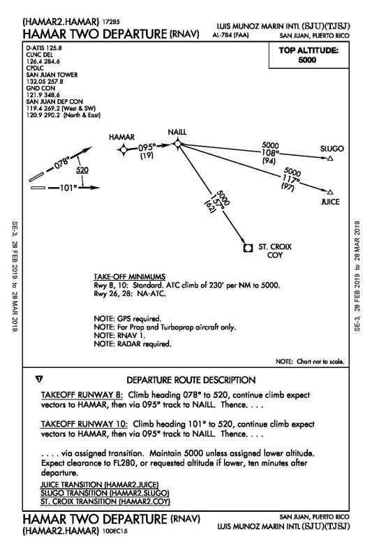
FIGURE 4-10 ALTERNATE HAMAR TWO DEPARTURE PROCEDURE
