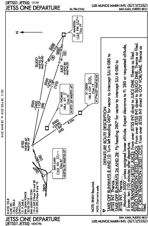
FIGURE 4-8 ALTERNATE JETSS ONE DEPARTURE PROCEDURE
