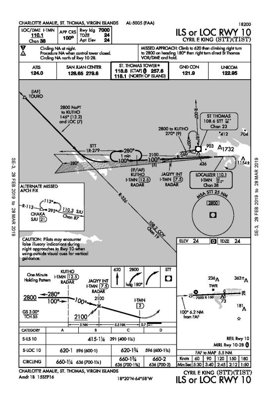
FIGURE 4-16 TOURO TO KUTHO INSTRUMENT APPROACH SEGMENT
