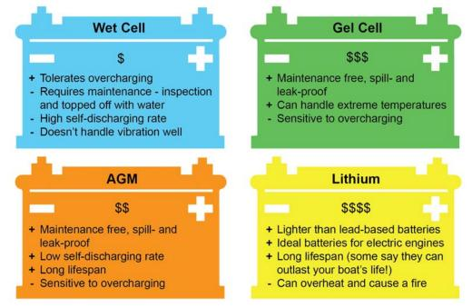
The most versatile type for marine use is the AGM battery. If you don't use your vessel daily, AGMs will hold their charge better than wet and gel cell batteries. Long lifespan and low self-discharge rate make AGM excellent dual-purpose (deep cycle and engine starting) batteries for boats.
