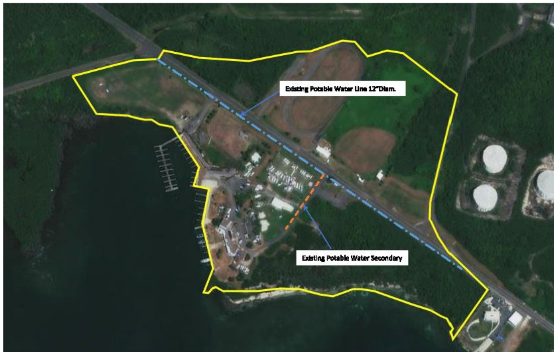
Exhibit I-1 Existing Potable Water Lines
