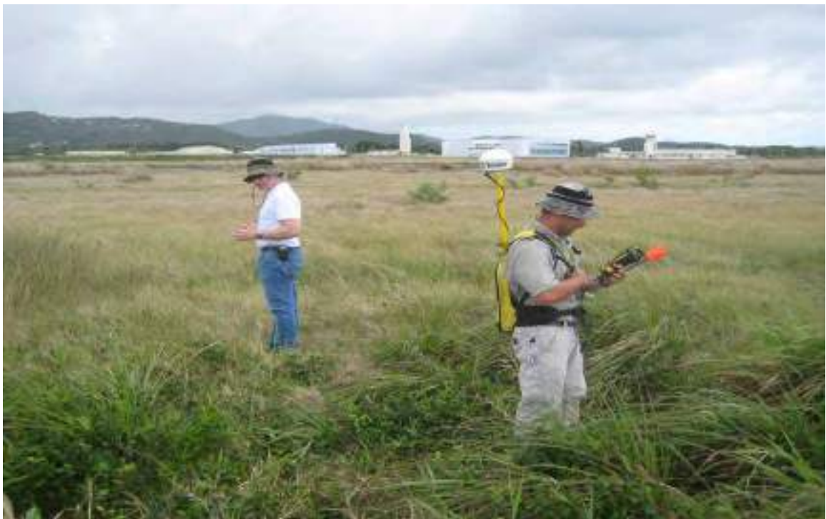
Baker associates locating soil boring and groundwater well locations using GPS
