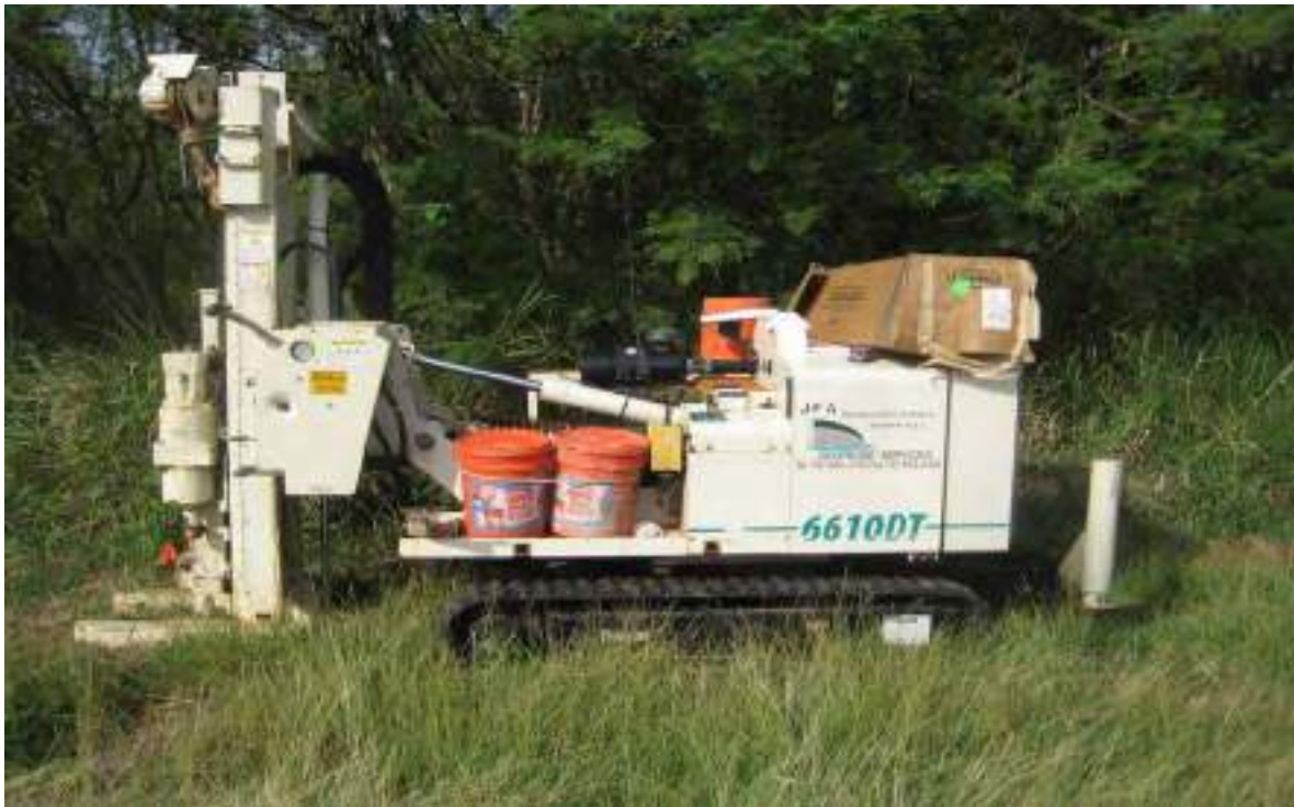
GeoProbe® Tracked Direct Push Machine operated by JFA Geological and Environmental Associates
