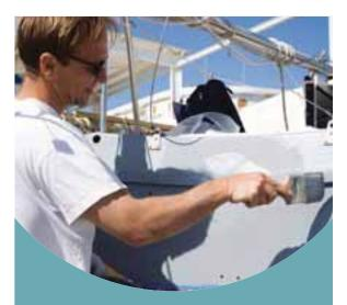
CONCERNED ABOUT THE HIGH LEVELS OF COPPER FOUND IN THE CITY'S MARINA BASINS, THE PORT OF SAN DIEGO TESTED AND EVALUATED THE EFFECTIVENESS OF VARIOUS NON-COPPER BASED ANTI-FOULING PAINTS ON MARINE VESSELS FROM 2008 TO 2010. THE RESULTS OF THIS STUDY WERE PUBLISHED IN A 2011 REPORT, "SAFER ALTERNATIVES TO COPPER ANTI-FOULING PAINTS FOR MARINE VESSELS."
