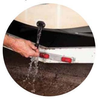
**Regularly inspect your boat's through-hull fittings** such as the depth finder transponder and cooling water intakes for leakage to reduce the risk of sinking. A sinking vessel not only poses a great safety risk to its passengers, but an unmanned vessel sinking at its dock or anchorage can introduce substantial amounts of fuel, oil and chemicals into the water.
