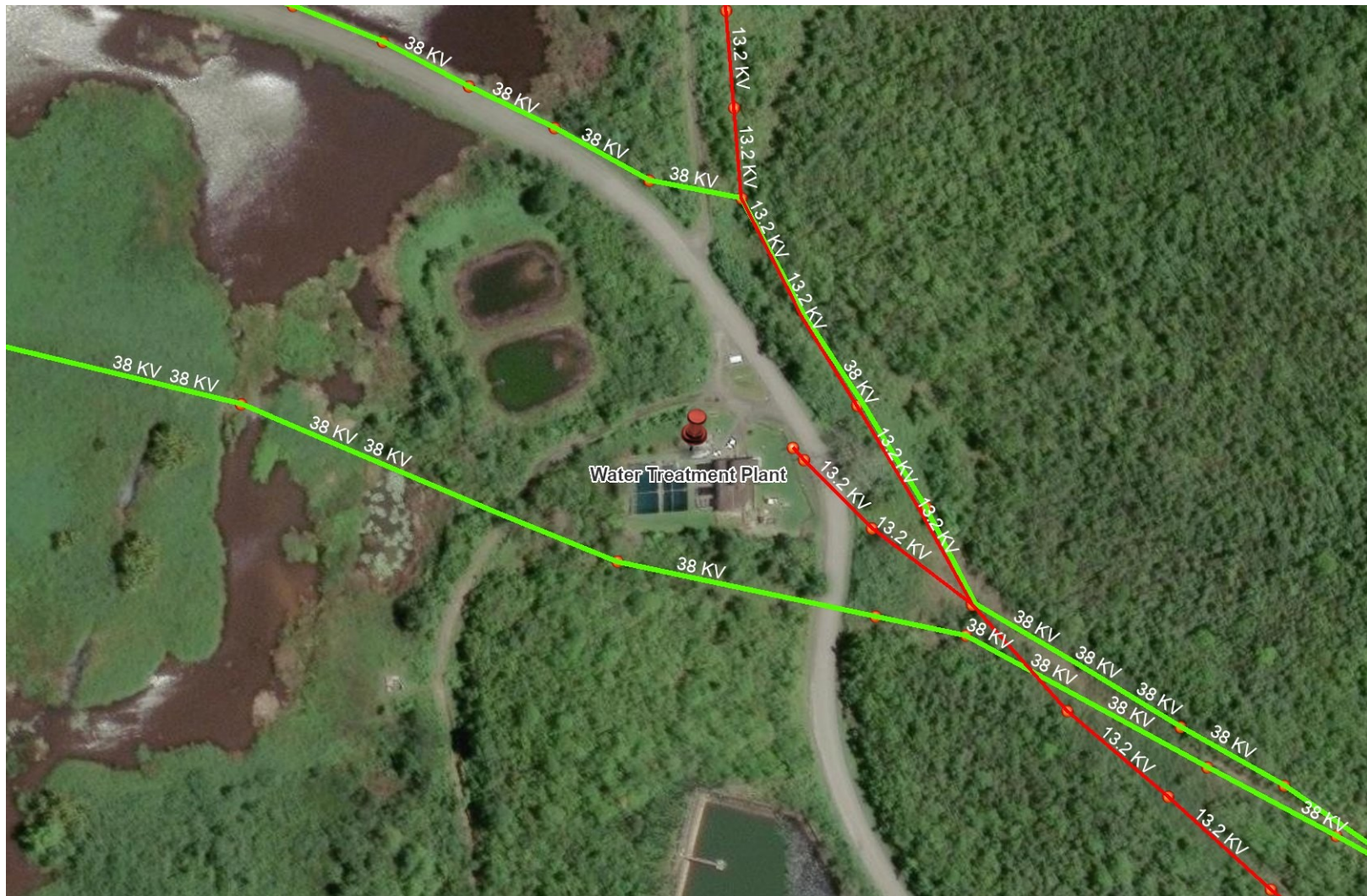
Figure 5. Water Treatment Plant – Electric Power Lines (for reference only)
