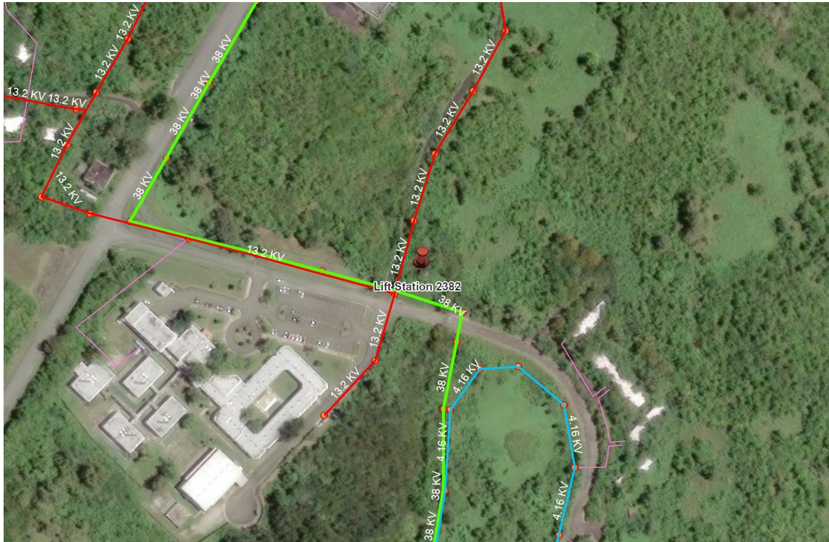
Figure 4. Lift Station 2382 – Electric Power Lines (for reference only)
